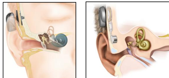
Fig. 3 BC implantable hearing aid Baha Bone Bridge
