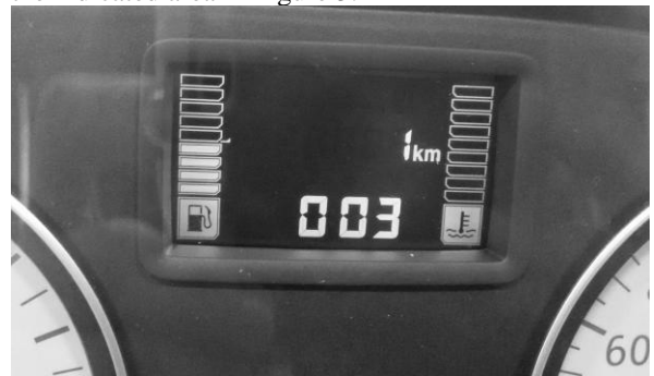
Figure 5 – The area which shows the level of fuel in the vehicle's tank on the dashboard's display.
