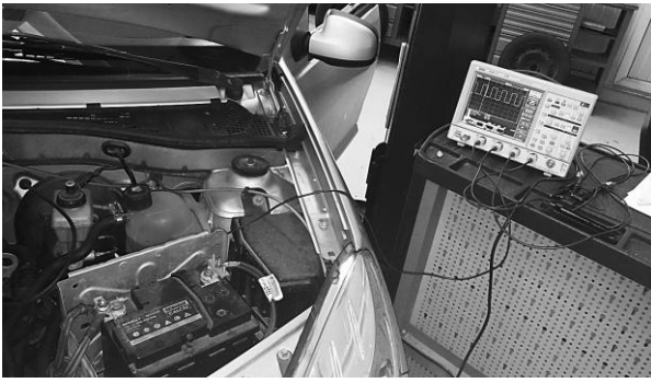
Figure 6 – ConsumedFuel parameter measurement from a Dacia’s Engine Control Unit, using the oscilloscope and varying the engine’s rotations / minute
