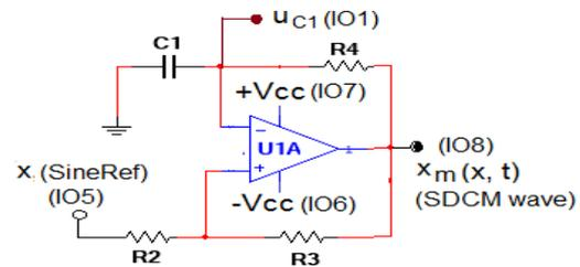
Figure 4. PWM circuit (No 2)
