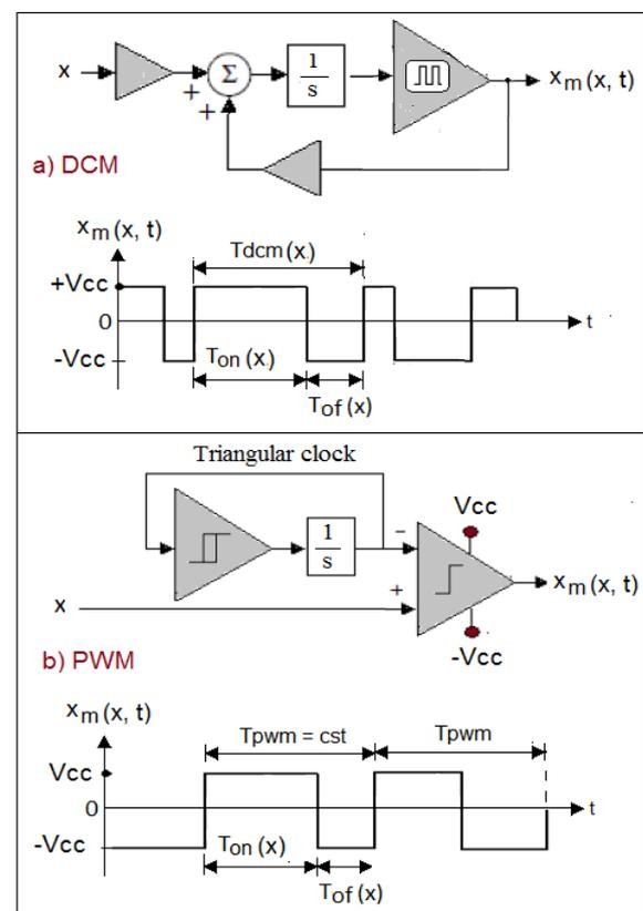
The principles of DCM and PWM drivers are recalled in Figure 1. Figure 1a shows that the DCM relies on a feedback loop structure, an embedded clock, and a modulated wave  $x_m(x, t)$  with modulation frequency  $f_m(x) = 1/T_m(x)$ , which evolves according to a given time varying profile, dictated by the modulating  $x$ . In Figure 1b, it is worth noting that the PWM relies on an open loop multistage architecture, due to the need of a triangular clock. In this case, the
