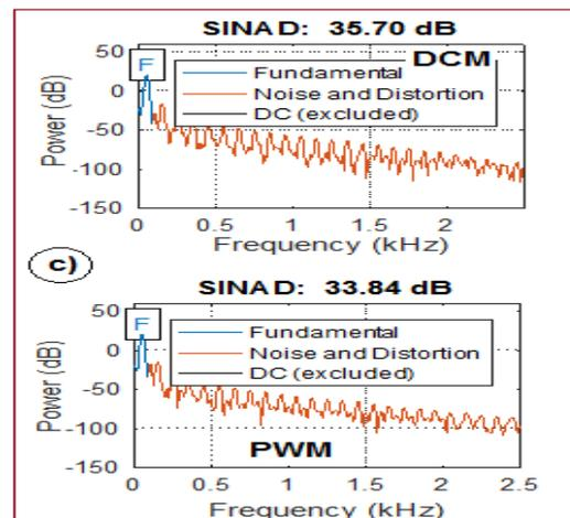
As a relevant finding, the normalized performances of the SDCM-based power inverter, are better in most cases than those of the SPWM-based architecture.
