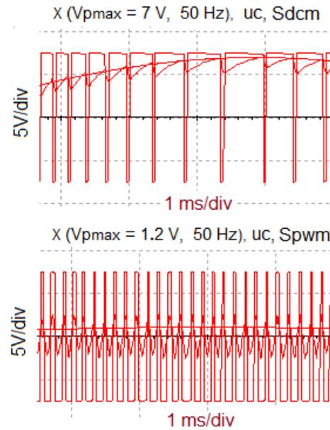
Figure 10. Transient time for SDCM and SPWM
