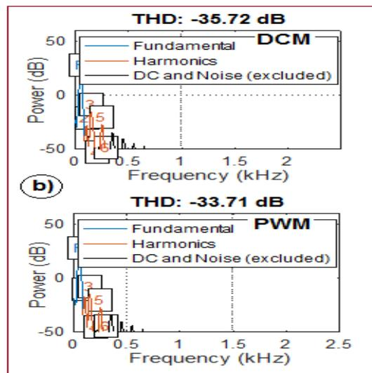
Figure 15. DCM-based and PWW-based SINADs
