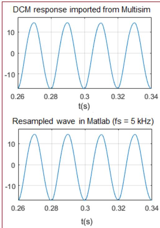
Figure 12. Multisim PWM data imported into Matlab and resampled version (at 5 kHz) using Matlab
