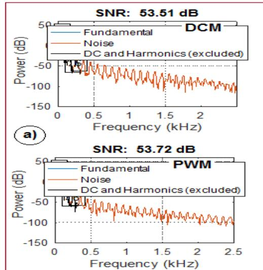
Figure 14. DCM-based and PWW-based THDs
