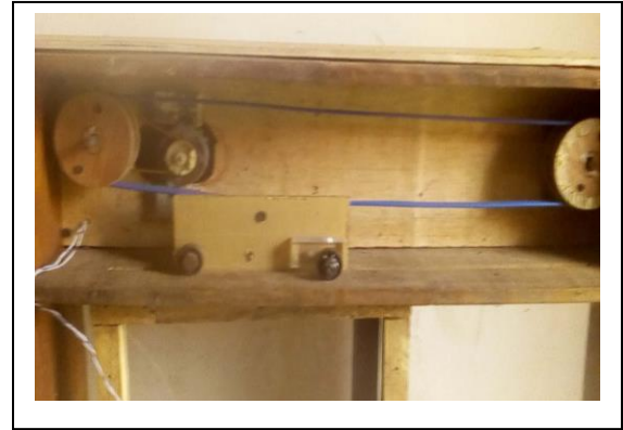
Figure 6. Pulley wheel to drive the sliding window
