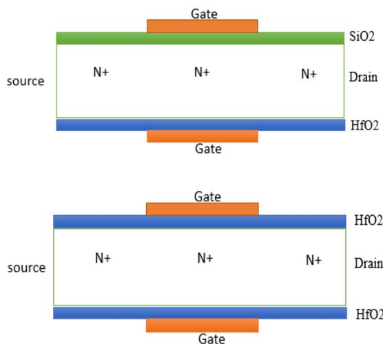
Figure. 2. Schematic device structures of symmetric and asymmetric oxide JLFET with an EOT value of 1 nm and Lch = 20 nm.
