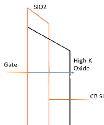
Figure. 1. Graphic of Direct tunneling through  $\text{SiO}_2$  and difficult tunneling through High-k Oxide ( $\text{HfO}_2$ ).
