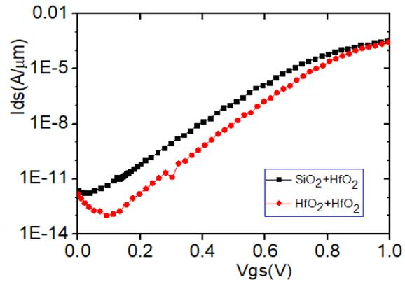
Figure.3. Measured output characteristics ( $I_{ds}$ - $V_{gs}$ ) of symmetric and asymmetric oxide JLFET ( $V_{ds}=1V$ )
