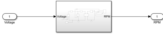
Figure 2.6: Block diagram of the acausal open-loop DC motor model (made in Matlab Simulink)
