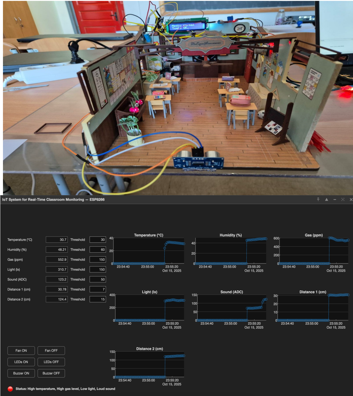
Figure 3. Integrated GUI and physical testbed of the ESP8266-based classroom environmental monitoring system
