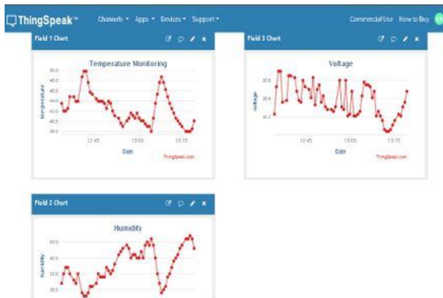
Figure 6. Real-time visualization of solar PV system parameters on ThingSpeak interface
