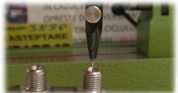
Figure 2. Gauge check of good piece
