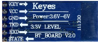
Figure 7. HC-05 Bluetooth pins
