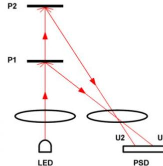
Figure 5. Infrared sensor operating principle
