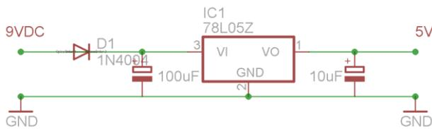
Figure 8. 9V to 5V C.C. voltage regulator schematic
