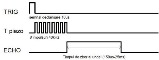
Figure 4. The operating principle of the ultrasonic sensor
