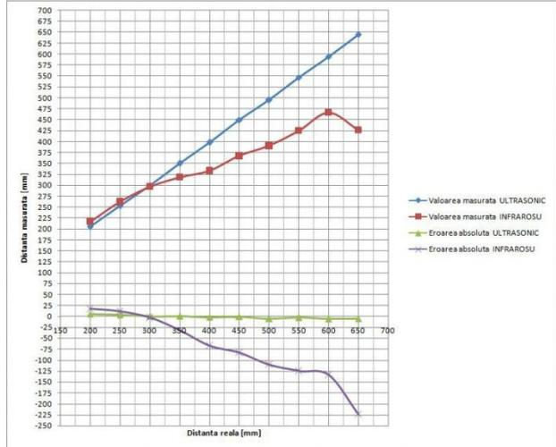
Figure 17. Graphic representation of results (metal)
