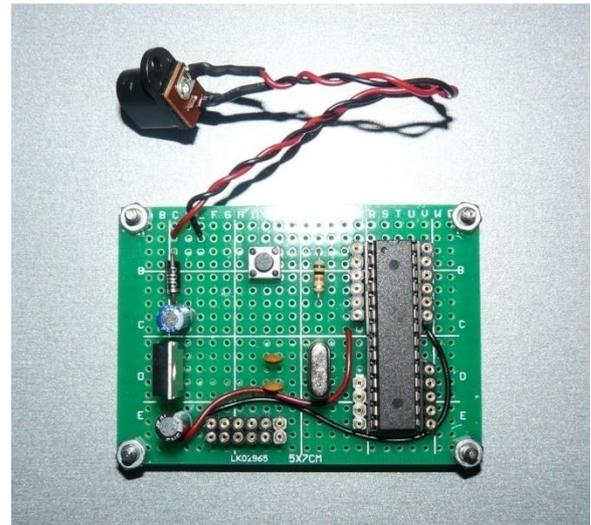
Figure 9. Base plate (CPU) after planting
