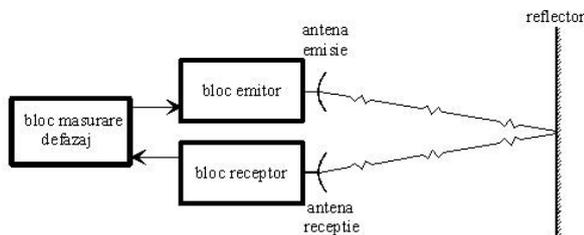
Figure 2. Measuring principle (wave propagation)
