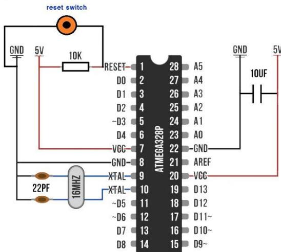
Figure 7. Mounting schematic and chip legend for ATmega 328P-PU
