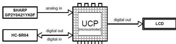
Figure 3. System Block Diagram
