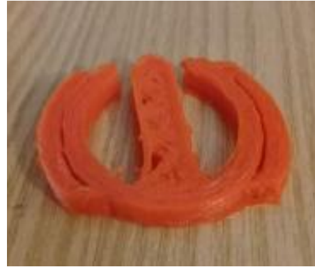
Figure 11. Printed logo of Hamdard University with slipped layers
