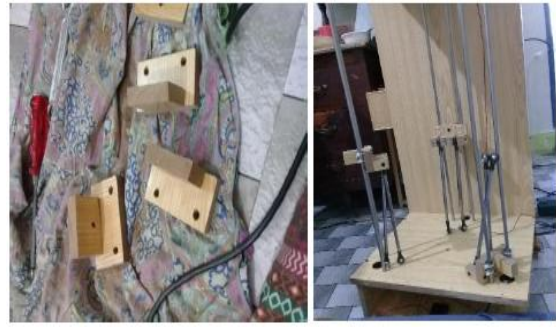
Figure 8. Wood rectangles for the supports of bearings
